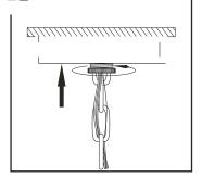
Carefully tuck wires into junction box and secure canopy to ceiling using screw collar ring.
