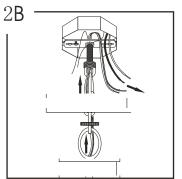
Slip screw collar ring and canopy onto chain, and hang fixture onto screw collar using an open link of chain.
