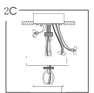
Strip 3/4?of insulation from wire ends. Connect house ground wire to fixture ground wire. Twist wires together using wire nut. Connect the black house wire to the smooth or black fixture wire. Twist wires together using wire nut. Connect the white house wire to the ribbed or white fixture wire. Twist wires together using wire nut.
