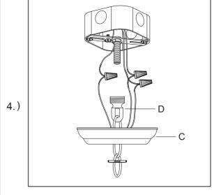
Step3:Install top loop to center stem and attach appropriate amount of chain to loop to achieve desired mounting height. Thread wire through every 3rd loop of chain.Remove ring from loop and slide down chain. Place canopy onto chain and let slide to top of fixture. Install nipple and cross bar into top of chain loop. Wire fixture to wires in outlet box. Copper wire is for Ground. Pull canopy through screw ring up chain to ceiling and tighten securely.
