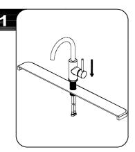
Optional Flange Installation: Before installation, place the faucet assembly through the mounting hole in sink
