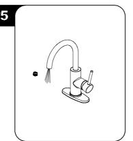
Important: After installation is completed, remove aerator. Turn on hot and cold water supplies. Turn handle to full open position for one minute. Check for leaks. Replace aerator.
