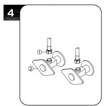
Make connections to water lines. Thread the nut (1) on the supply line onto the outlet of the water supply valve (2) and tighten with a wrench. Do not overtighten.
