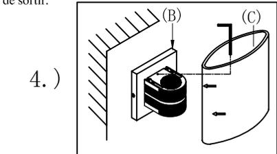
Step 4: Snap the shade (C) over the light engine (B) on the fixture and secure with Allen screw.
