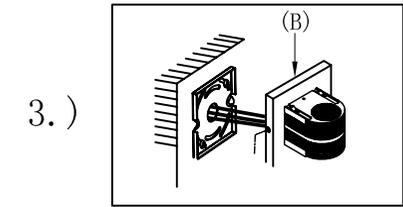
Step 3: Place the fixture on the back plate, and secure with two screws on the sides to hold the fixture in place. Caulk around back-plate where fixture meets the wall using outdoor silicone sealant. Leave a small gap at the bottom to allow moisture to escape.
