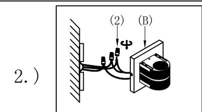
Step 2: Use wire nuts supplied to wire fixture to wires in outlet box. Copper wire is for Ground.
