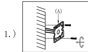
Step 1: Remove mounting bracket from fixture (B) and install to electrical box.
