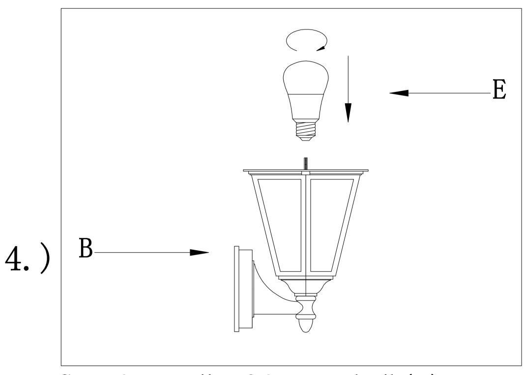
Step.4: Install E26 LED bulb(E)
