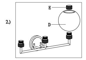
Step 2. Attached the glass(D) on the socket then secure by socket ring(E).
