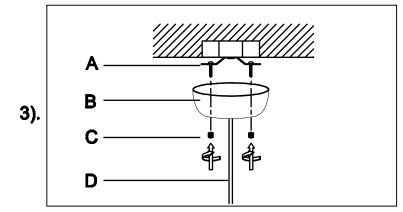
Step.3: Adjust cable length to desired mounting height, and tighten strain relief screws to secure. Install body(C) tobracket(A) and tighten finials(C) on the canopy(B) to secure.
