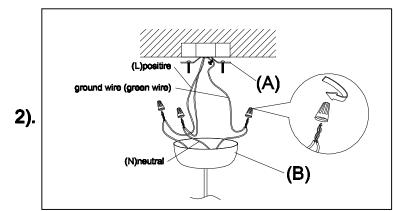
Step.2: Wire fixture to wires in outlet box.
