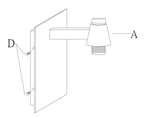
2. Caulk around backplate where fixture meets the wall leave a hole at the bottom to allow water to escape.
