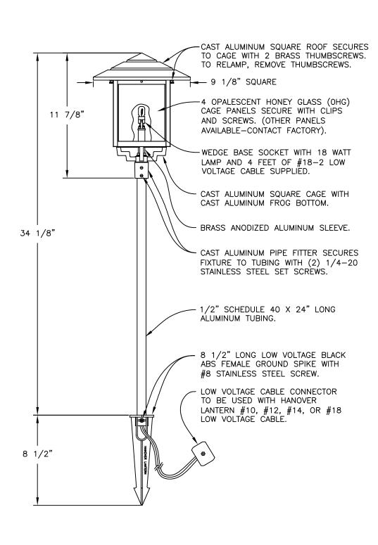
LANTERN WILL BE PREWIRED AND TESTED. ELECTRICAL COMPONENTS ARE U.L. LISTED. ALL MOUNTING HARDWARE IS SUPPLIED.
