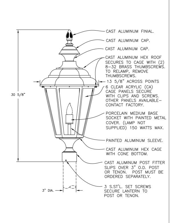
LANTERN IS PREWIRED AND TESTED. ELECTRICAL COMPONENTS ARE U.L. LISTED. MOUNTING HARDWARE IS SUPPLIED.
