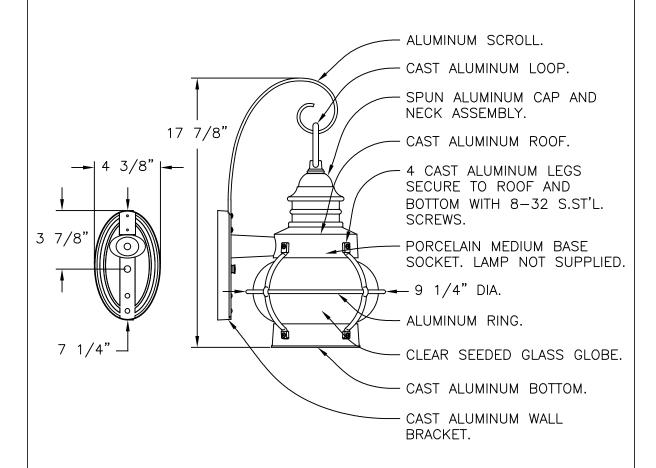
LANTERN WILL BE PREWIRED AND TESTED. ALL ELECTRICAL COMPONENTS ARE UL. LISTED. MOUNTING HARDWARE SUPPLIED.
