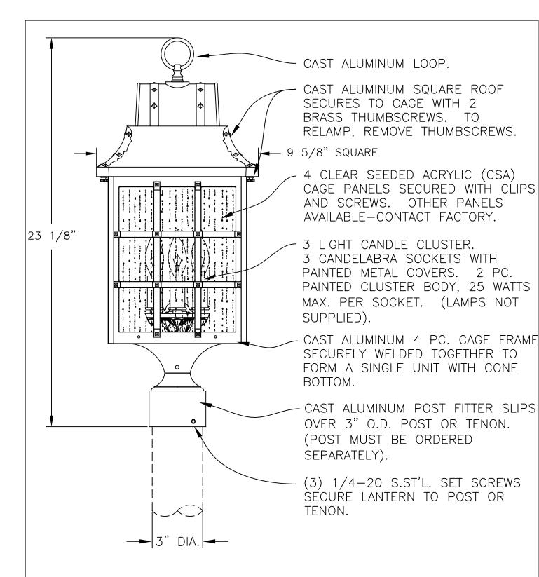
LANTERN WILL BE PREWIRED AND TESTED. ALL ELECTRICAL COMPONENTS ARE U.L. LISTED.
