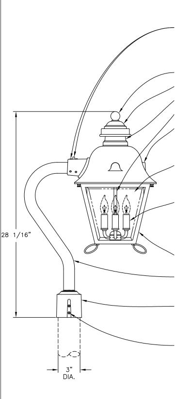
STAINLESS STEEL DRIVE PIN TO LOCK LANTERN TO ARM WITH (6) 1/4-20 STAINLESS STEEL SET SCREWS TO LEVEL AND SECURE LANTERN TO ARM.
