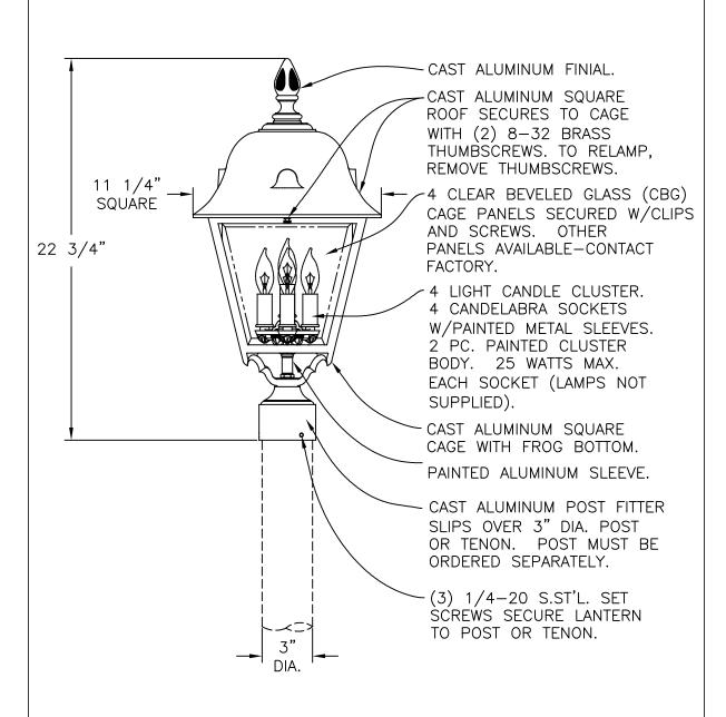
LANTERN IS PREWIRED AND TESTED. ELECTRICAL COMPONENTS ARE U.L. LISTED. MOUNTING HARDWARE IS SUPPLIED.
