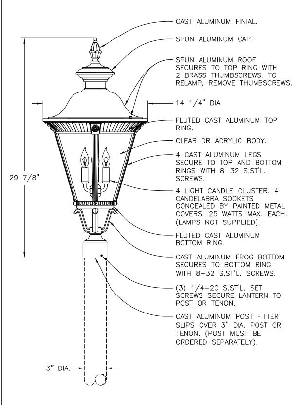
LANTERN WILL BE PREWIRED AND TESTED. ALL ELECTRICAL COMPONENTS ARE UL. LISTED. MOUNTING HARDWARE SUPPLIED.
