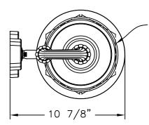
LANTERN TO BE ASSEMBLED AS SHOWN IN TOP VIEW—MOUNTED ACROSS FLATS.
