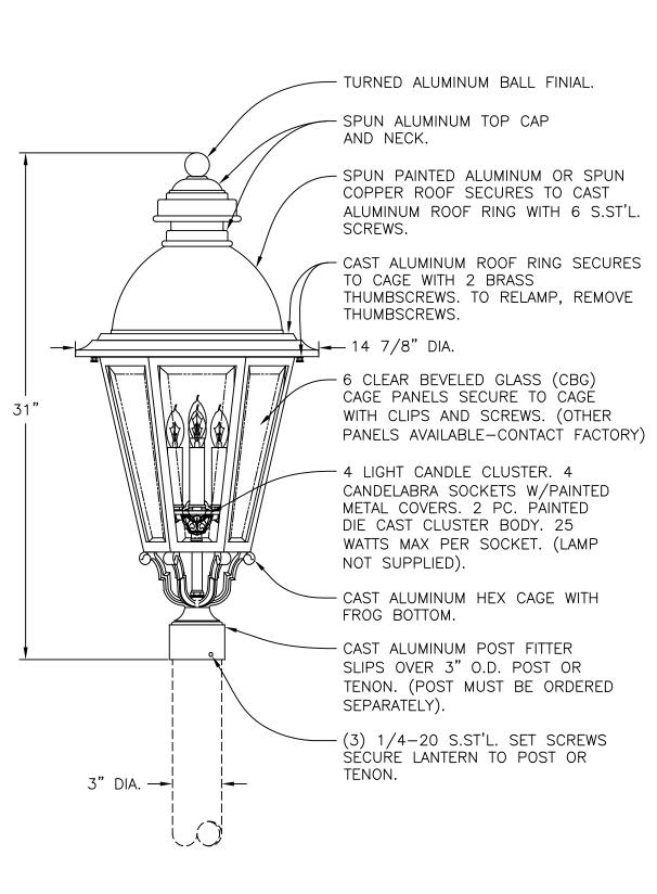
LANTERN WILL BE PREWIRED AND TESTED. ALL ELECTRICAL COMPONENTS ARE U.L. LISTED. ALL MOUNTING HARDWARE SUPPLIED.
