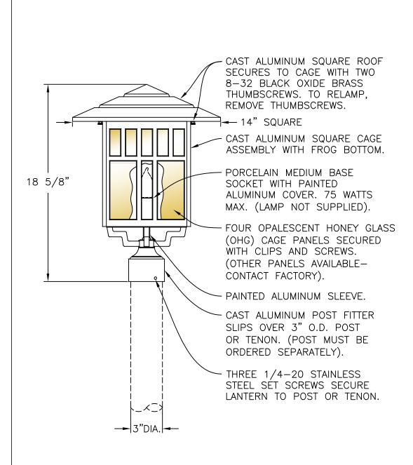
E.P.A. = 0.82 (EFFECTED PROJECTED AREA). LANTERN WILL BE PREWIRED AND TESTED. ALL ELECTRICAL COMPONENTS ARE U.L. LISTED. ALL MOUNTING HARDWARE IS SUPPLIED.
