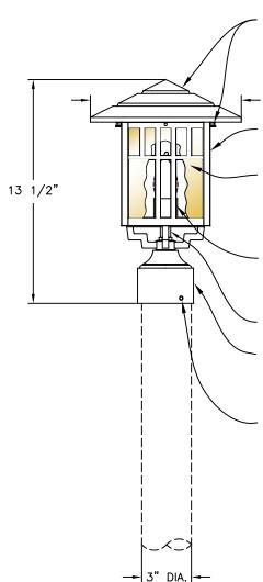
CAST ALUMINUM SQUARE ROOF ATTACHES TO CAGE WITH TWO BLACK OXIDE BRASS THUMBSCREWS. TO RELAMP, REMOVE THUMBSCREWS.
