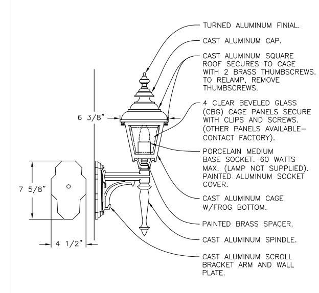
LANTERN WILL BE PREWIRED AND TESTED. ALL ELECTRICAL COMPONENTS ARE U.L. LISTED. ALL MOUNTING HARDWARE SUPPLIED.
