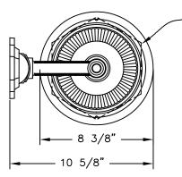
LANTERN TO BE ASSEMBLED AS SHOWN IN TOP VIEW— MOUNTED ACROSS FLATS.
