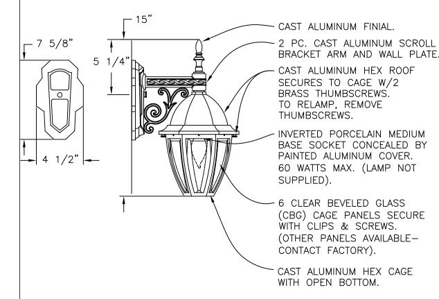
LANTERN WILL BE PREWIRED AND TESTED. ALL ELECTRICAL COMPONENTS ARE UL. LISTED. MOUNTING HARDWARE SUPPLIED.
