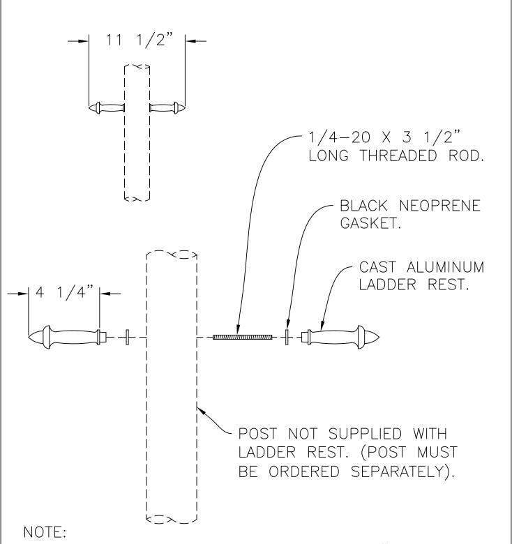
MOUNTING HARDWARE IS SET UP FOR A 3" DIA. POST. ALL MOUNTING HARDWARE IS SUPPLIED AS SHOWN.
