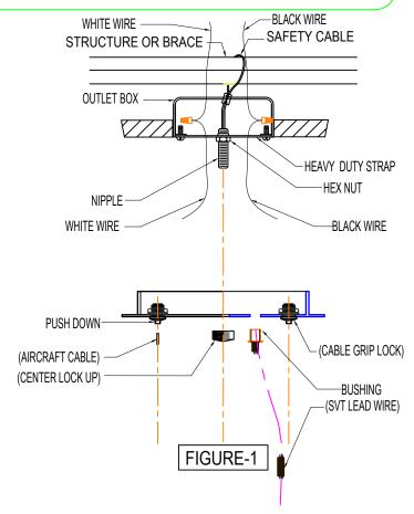
5. Attach the heavy duty strap to the outlet box using the mounting screws. Attach the safety cable to the building structure or brace.(Refer Figure-1).
