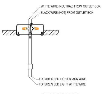
LED LIGHT TO OUTLET BOX WIRE CONNECTION DETAILS
