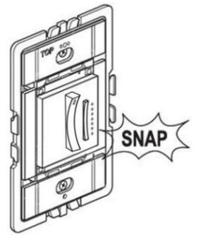
**NOTE - If you need to remove a device from the frame, remove frame from wall box. Insert a flat screwdriver from the back of the frame and depress the tabs on the device to unlock and push it forward.**
